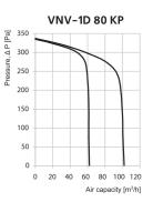
The abrupt curves show high pressure performance of VNV fans and constant air flow while operation of many fans integrated into single ventilation
